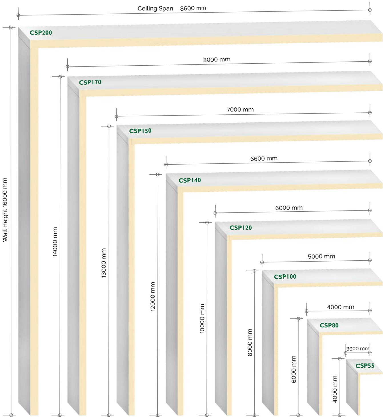
\* Span table is based on panels with 0.50mm thick steel internal and external facers
